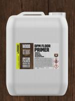
WOODSTIKK®DPM FLOOR PRIMER IS A ONE COMPONENT SOLVENT-FREE POLYURETHANE PRIMER COATING WHICH IS USED FOR SUPPRESSING RISING DAMP AND RESIDUAL CONSTRUCTION MOISTURE IN SUBFLOORS PRIOR TO BONDING WOOD FLOORING DOWN. IT CAN ALSO BE USED FOR PRELIMINARY TREATMENT OF SANDY OR POWDERY SUBFLOORS.
